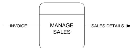
6. No process should be there in the DFD, which has only incoming edges. If the process has only incoming edges and no outgoing edge then it is called a problem Black hole.
