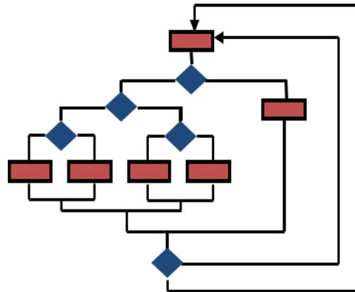
A small C program contains two nested loops that execute from 1 to 20 times each depending on input. There are 4 if-then-else constructs inside the inner loop as given in the flow chart.
