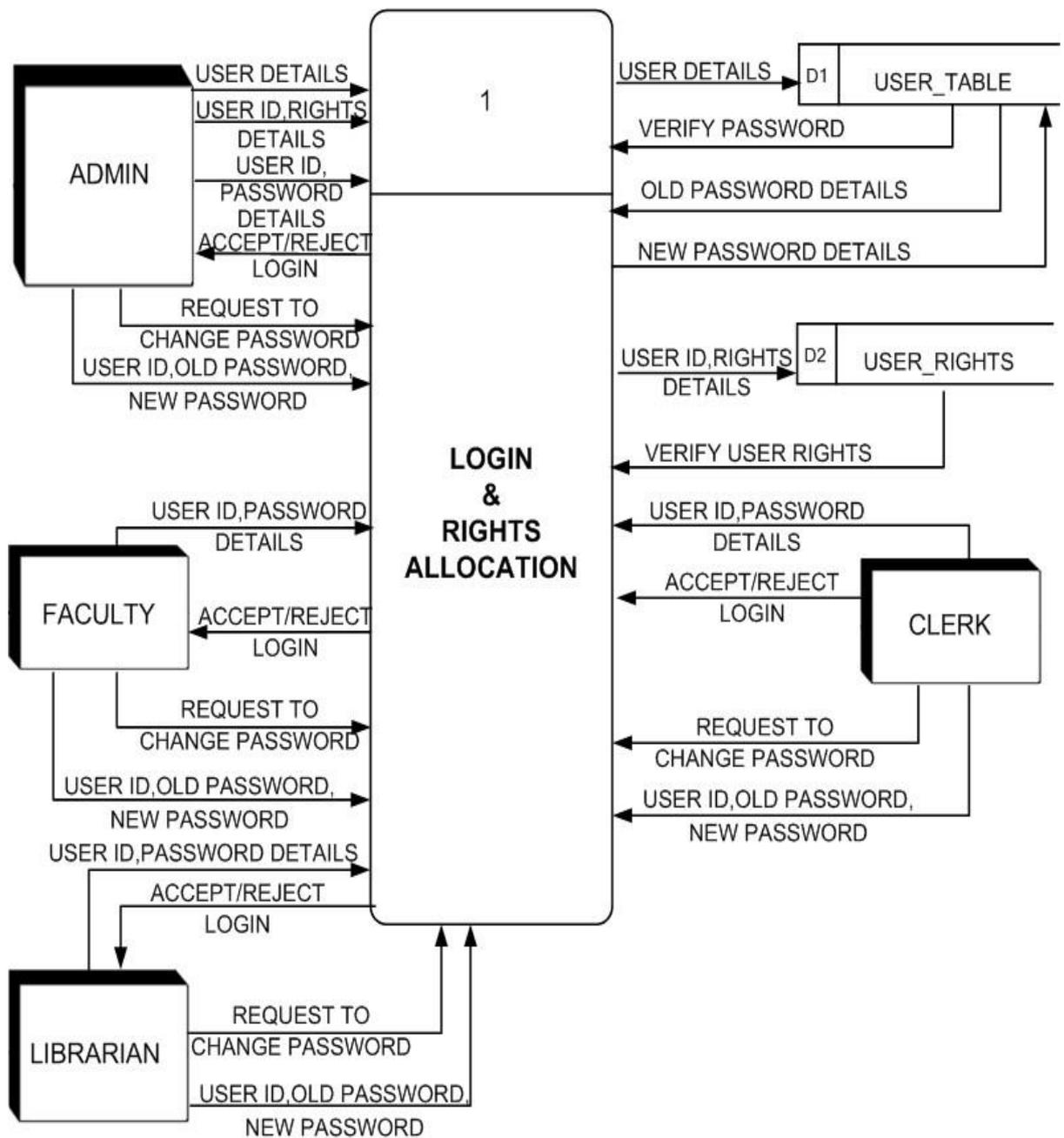
This is the 1<sup>st</sup> process of the 1<sup>st</sup> Level DFD. Different users can log into the system and based on their role system will give privileges to the user. The process is complex and its 2<sup>nd</sup> level decomposition is required. Its 2<sup>nd</sup> level DFD is represented in the next figure.
