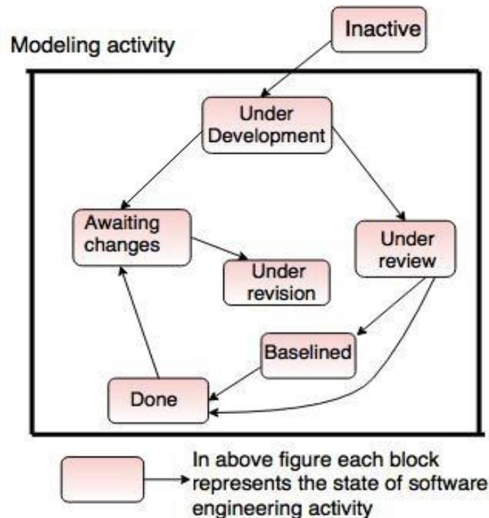
**Figure-10 One Element of Concurrent Process Model**
