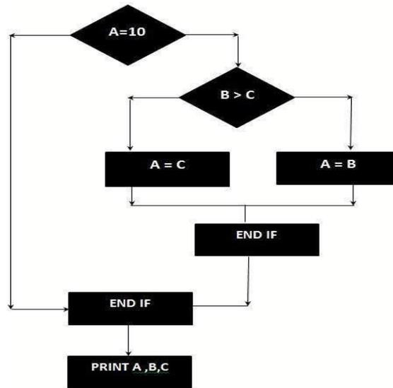
For examples, the control flow diagram shown above have seven nodes (shapes) and eight edges (lines), hence the
