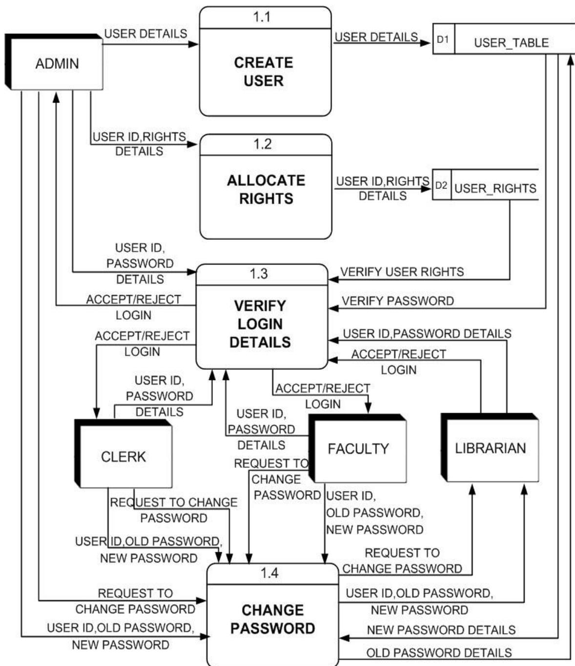
Here the whole login process we have decomposed into Create user, Rights allocation, Verify login (Authentication) and Change password. Our next process is to record details for all our master tables in the database. The process is simple enough, hence second level transformation is not needed.
