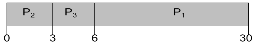
Figure 2.3: Sample arrangement of process in SJF scheduling
